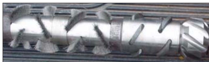
Various tools provide a means for mechanically cleaning the casing. The top photo shows a casing brush-scraper combination. The middle photo is a closeup of a set of scrapers and two sets of brushes on one tool. The bottom photo shows a riser brush (Fig. 5).
