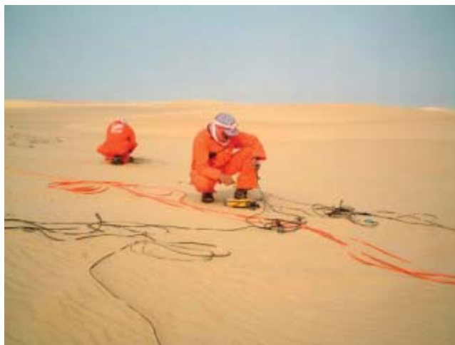
Cableless land acquisition is seen as having the potential to significantly reduce land acquisition costs. An onshore seismic crew is shown laying out cables with sensors in the desert. Photo courtesy of Petroleum Geo-Services ASA.
